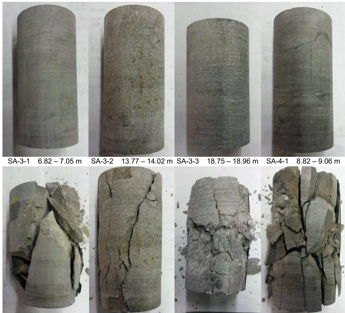
Figure 4: Photographs of test specimens before testing (top) and after testing (bottom).
