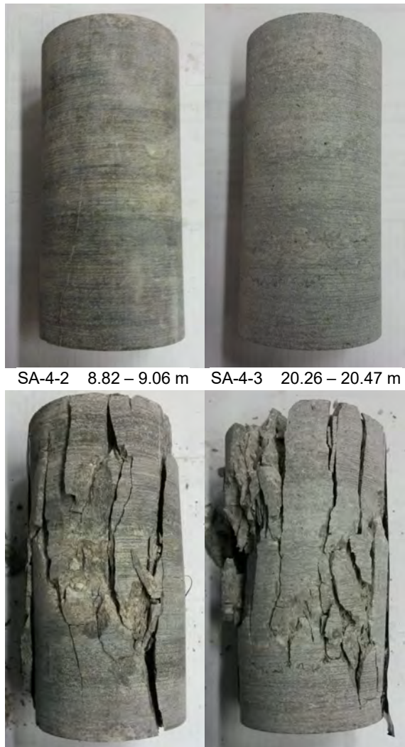
Figure 5: Photographs of test specimens before testing (top) and after testing (bottom).
