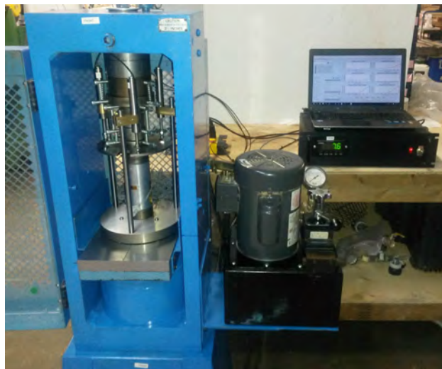
Figure 1: Forney loading frame used for uniaxial compression testing.
