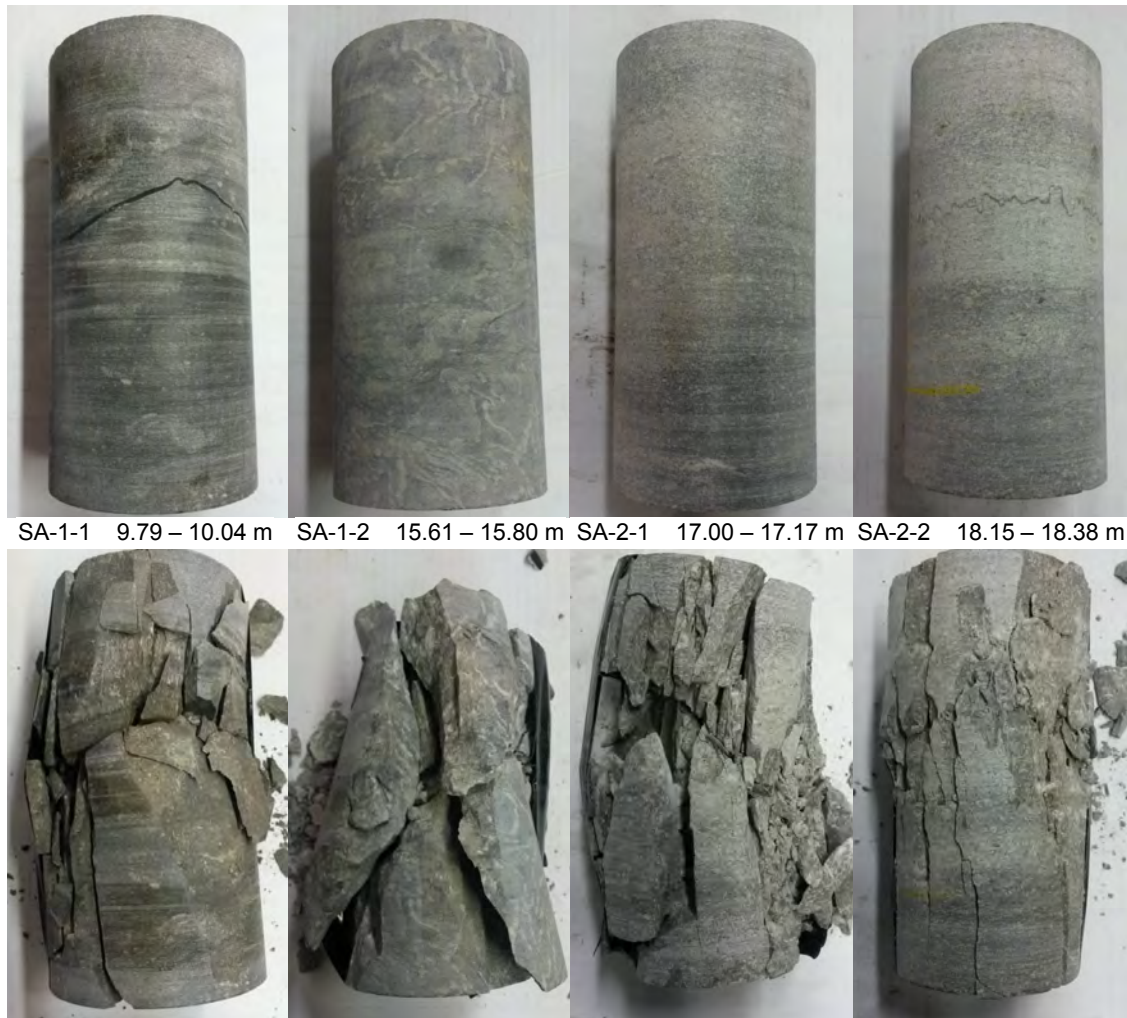
Figure 3: Photographs of test specimens before testing (top) and after testing (bottom).
